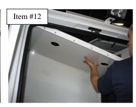
Position 3<sup>rd</sup> Compartment Ceiling into vehicle.
